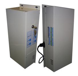
A wall- or rack-mounted 24 V DC battery-backed power supply that is compatible with the TACERA Nurse Call System. It operates on 110-240 V AC input via a fuse-protected mains input socket and cable.
