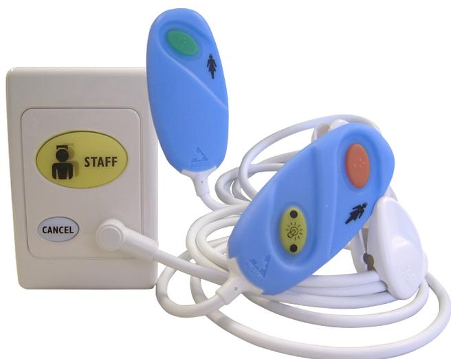
An ergonomically designed, easy-to-grip pendant for patients to activate calls on a TACERA Nurse Call System. The solid blue, water resistant case is non-slip and dip sterilisable, and is available with or without patient control of lights. The soft touch buttons are recessed to avoid accidental activation. The entire pendant is manufactured from silicone rubber with an anti-bacterial additive for improved infection control.
