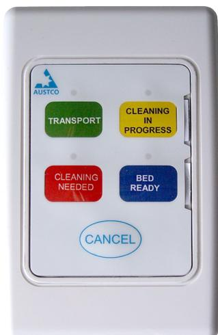
A flush wall-mounted callpoint that is used for both Nurse Call and Workflow applications. The 4 touch buttons can be individually programmed, locally or remotely, for any Nurse Call, Status or Workflow function. Each button has a user-inscribable tag that indicates its function and is placed behind a clear lexan cover for improved infection control.
